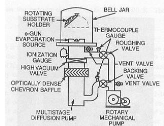
Figure 2-12. Schematic of vacuum deposition system.
